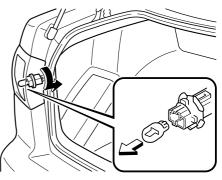
5. Install the new bulb in the reverse order of removal.
